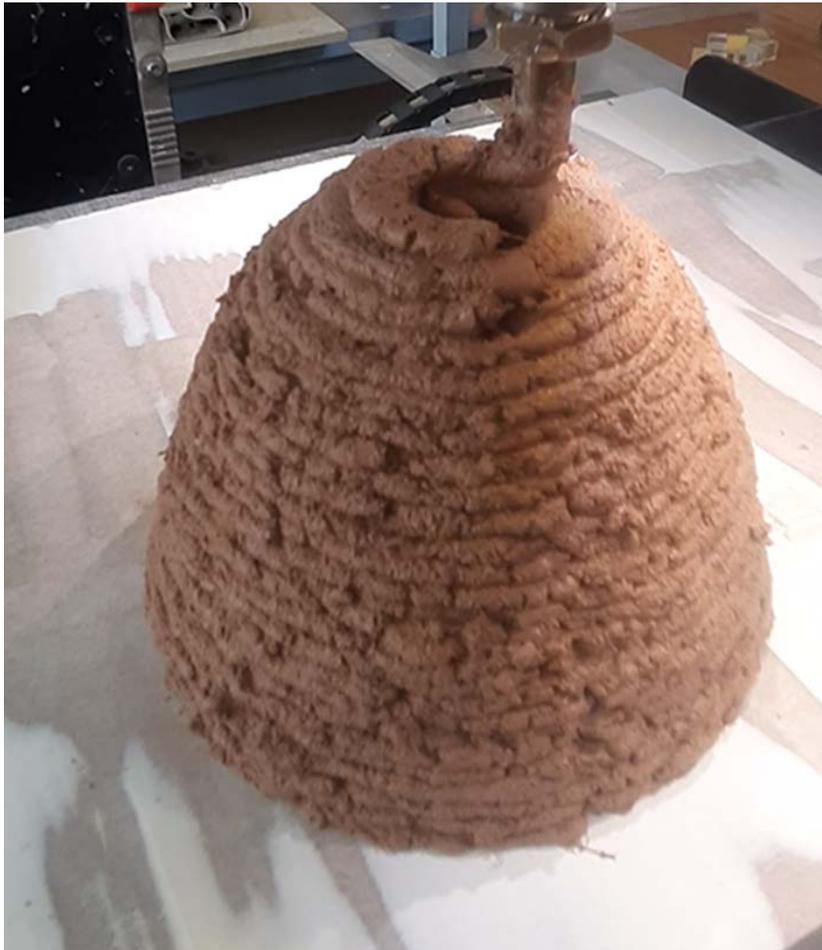
Extrudability test of earth based composite consist of earth(ecoclay) + straw natural fiber + sodium silicate binder + water + fine sand.
