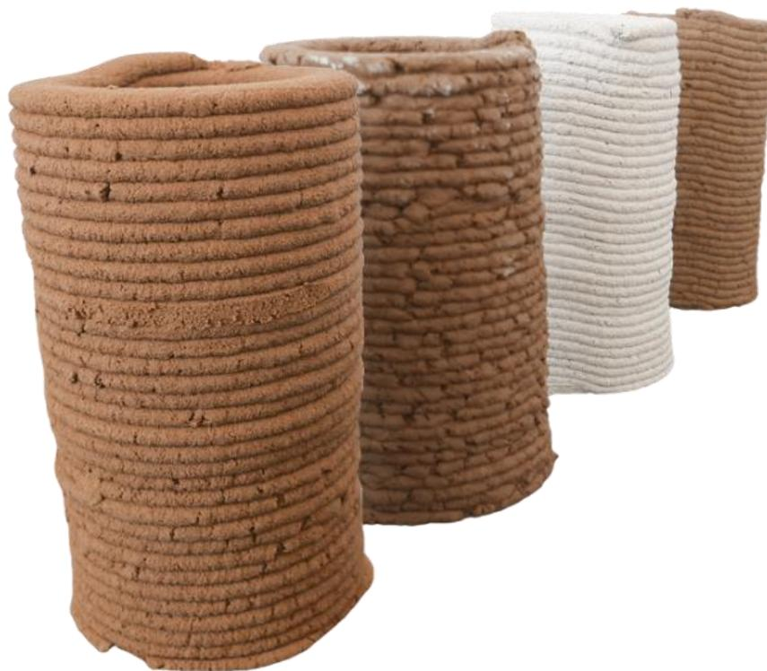
*Figura 8. Additive manufacturing of Earth-based composites by considering different Ingredients In the material matrix to improve the physical and mechanical properties.*
